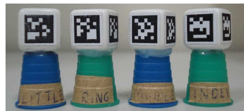
Figure 3. Dices with ARToolkitPlus patterns. Since the thumb is not taken into account in the current data glove prototype, there are only four dices.
